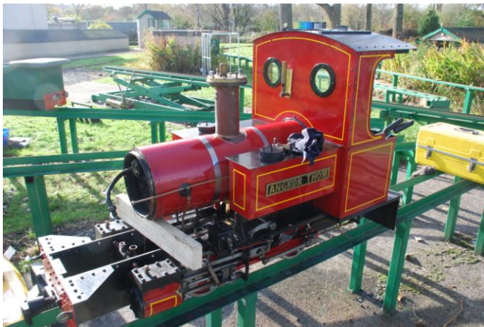
Left – Dave Henderson's "Ankor Thom", minus smokebox, having a boiler leak inspected. Right – Ray Simpson's Regner 16mm scale Guinness Tram
