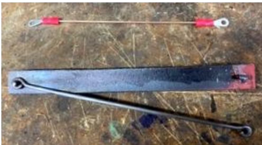
Photo showing the wire with crimped eyelets, the jig and the wire tie rod made on the jig.
